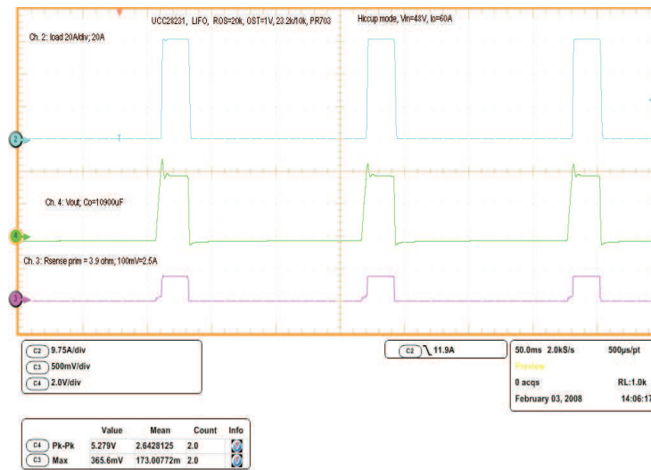
Figure 42. Cycle-by-Cycle Current Limit
